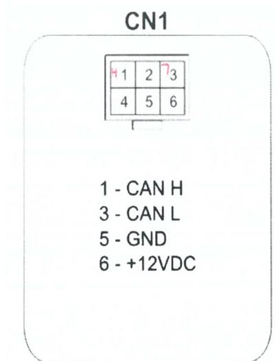
Fig. 1: Display's connection scheme
