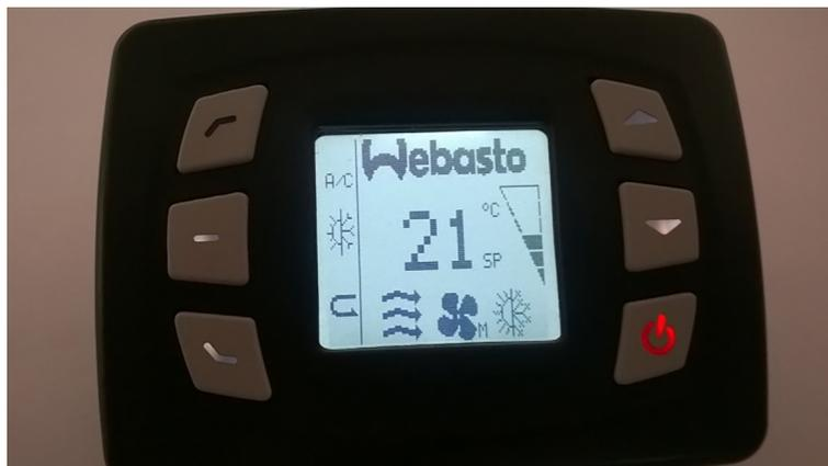
Fig. 5: Auto Mode, Manual Fan Speed
